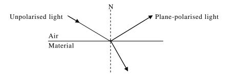
The reflected light is plane polarised. Sketch the diagram and write in the values of all the angles.
