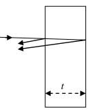
The two reflected rays can interfere constructively or destructively.
