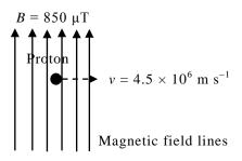
Calculate the magnetic force exerted on the proton.
