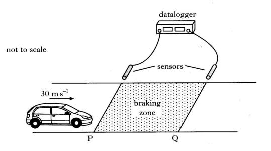
The sensors are connected to a datalogger which records the speed of the car at both P and Q.
