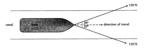
Each rope exerts a force of 150 N at 20° to the direction of travel of the boat as shown.
