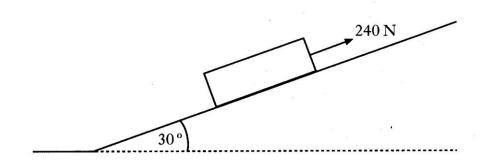
A force of 240 N is applied to the crate parallel to the slope. The crate moves at a constant speed of  $3.0 \text{ m s}^{-1}$ .
