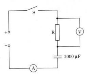
The graphs below show how the potential difference  $V_{\rm R}$  across the **resistor** and the current I in the circuit vary with time from the instant switch S is closed.
