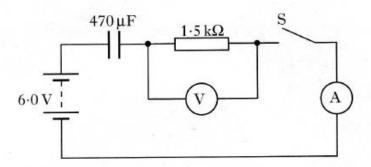
The capacitor is initially uncharged.
